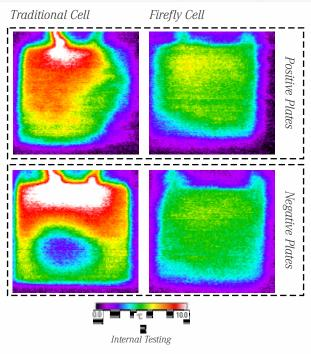
Infrared thermal images snapped at the end of a 5C (12 minute) discharge of both a Firefly 3D cell and a Traditional cell.
