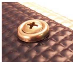
Solara Walk-On solar panels can also be screwed down, and the encapsulated backing plate is pre-drilled with holes for this purpose. Use a 3/16" drill to penetrate the front and rear coating at the locations of the pre-drilled holes, then screw the panel down with stainless steel screws and finishing washers. Do not drill or attempt to drill any additional holes in the panel. Only use the pre-drilled fixing points to secure a panel with screws.
